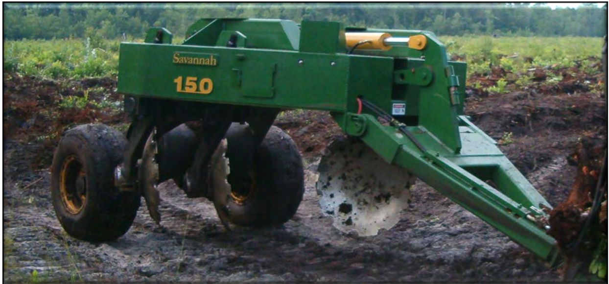
The Magnum™ 150 trailing plow provides Complete Cultivation under the planting zone by using an inner disk set to cultivate directly under the planting zone of the seedling.
